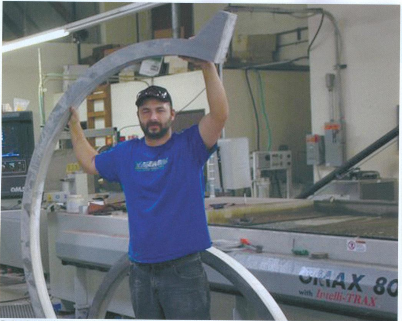
TruPart Manufacturing owner Shane Prukop stands among 3-inch thick aluminum parts cut by an OMAX 80X JetMachining Center. All components, made for an aerospace client, were cut within seven hours.
